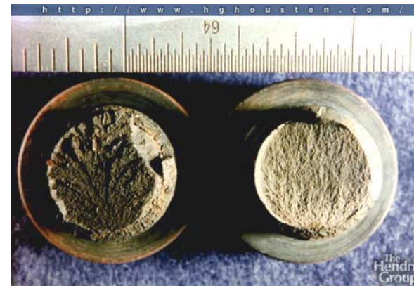
Hydrogen Embrittlement of Valve Capscrew Fasteners
