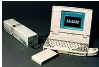
A Ballard fuel cell powers a laptop computer.
