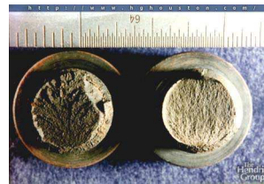
Hydrogen Embrittlement of Valve Capscrew Fasteners
